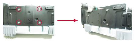
Remove the 4 screws attaching the bag to the bottom of the device.
