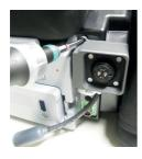
Now, fasten the LP15 Power Adapter to the device. To do so, please use the screws that were used to fasten the cover over the USB port.
