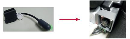
Take the LP15 Power Adapter and place it on the USB port as shown in the image above. Ensure that the Adapter is sitting cleanly on the port, as it can easily become tilted in the bag.
