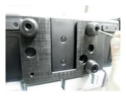
Place one of the included washers into each of the provided plastic feet, then use the pro-vided screws to screw the Adaptation w/o power onto the bottom of the device.
