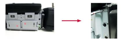
Remove the cover over the USB port on the back of the device. Do not lose the screws, as they are needed in a later step. Please also store the cover carefully for later use.
